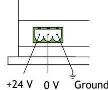
*Maximum length of 24 V DC power supply cable is 10 meters.*
